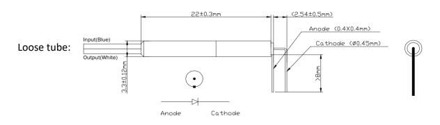
Anode is connected to the metal housing.
